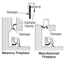
Figure 9 - Attaching Damper Clamp
